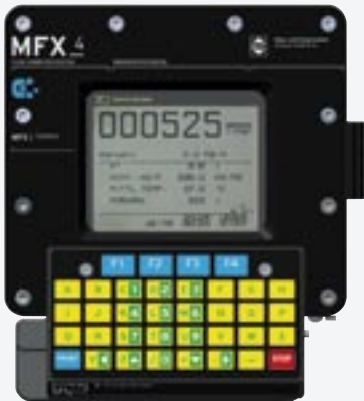
MFX_4 Terminal is the Human-Machine-Interface Module
